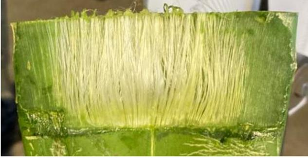
A cross-section of a leaf after 6 impacts with a 0.6 mm calibration. The fibers are poorly separated, appearing as a dense, somewhat clumpy mass of green and yellowish strands. |
