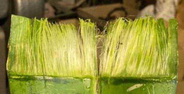
A cross-section of a leaf after 13 impacts with a 0.4 mm calibration. The fibers are more clearly separated into distinct bundles, showing a regular pattern.                   |
