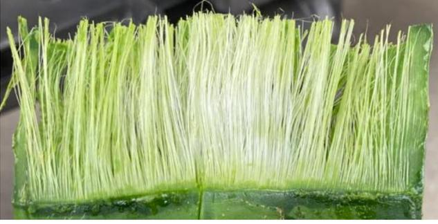
A cross-section of a leaf after 15 impacts with a 0.2 mm calibration. The fibers are very well separated, appearing as numerous fine, distinct strands.                        |
