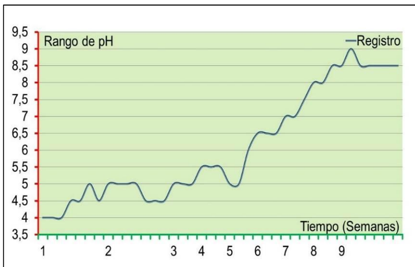
Figura 12: Control de pH del abono compost.
