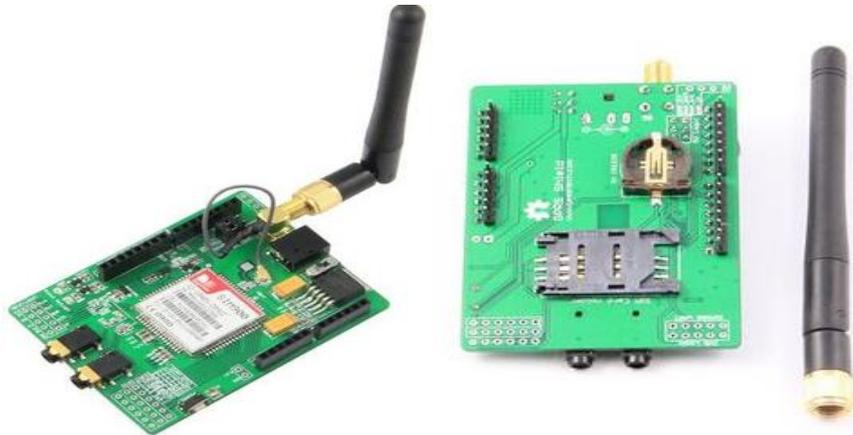
The GPRS Shield is based on SIM900 module from SIMCOM and compatible with Arduino and its clones. The GPRS Shield provides you a way to communicate using the GSM cell phone network. The shield allows you to achieve SMS, MMS, GPRS and Audio via UART by sending AT commands (GSM 07.07, 07.05 and SIMCOM enhanced AT Commands). The shield also has the 12 GPIOs, 2 PWMs and an ADC of the SIM900 module (They are all 2V8 logic) present onboard.
