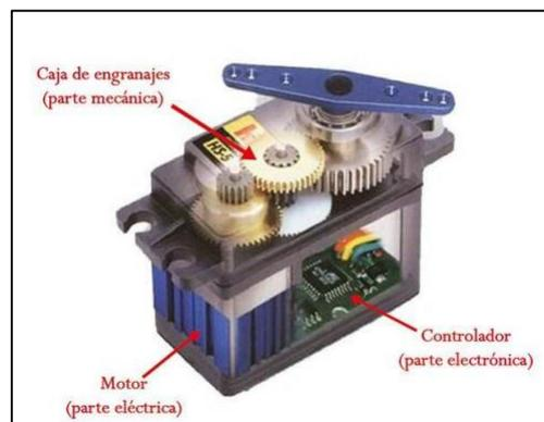
**Figura 16.** Servomotor.
