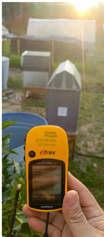
**Figura 57.** GPS portátil Garmin eTrex Venture HC
