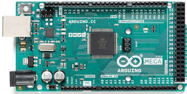
**Figura 24.** Arduino Mega 2560.
