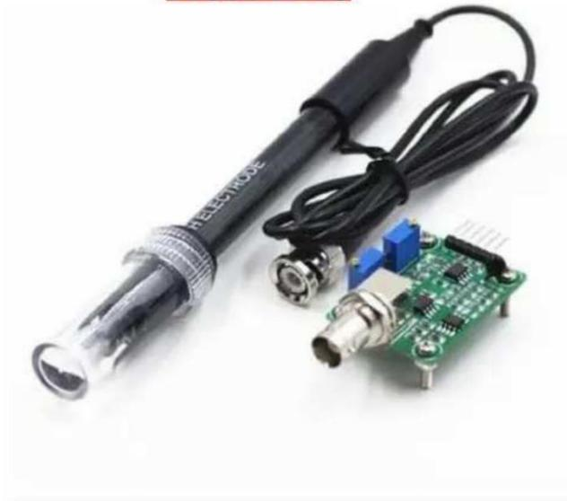
The PH sensor is a low-cost, easy-to-use PH meter detection sensor. This sensor module can be used as an analog PH meter designed by Arduino, MCU and other controllers. It has the characteristics of simple connection, convenient and practical.
