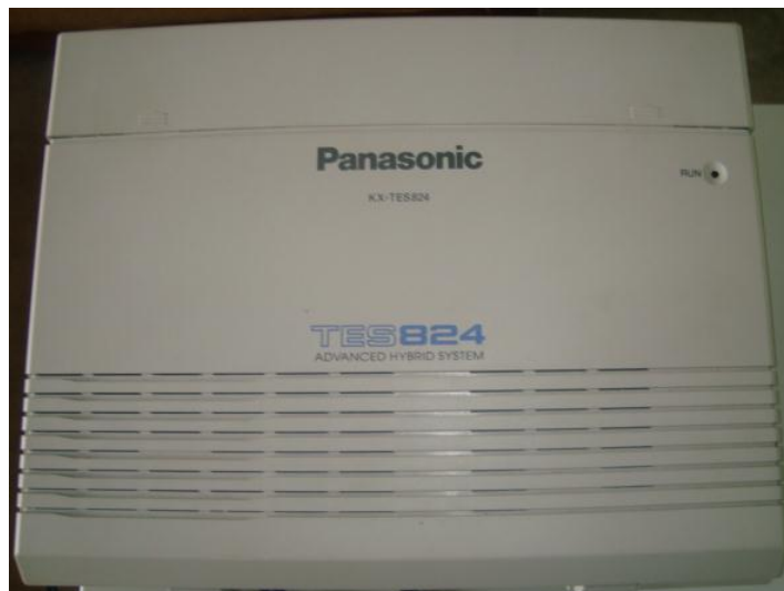
Fig.4 Centralilla telefónica Panasonic KX-TES824
