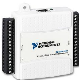
Fig.2.11 Tarjeta DAQ NI USB-6008 de National Instruments
