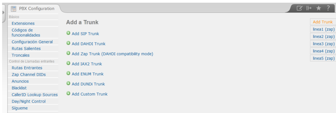
Figura 49. Agregar troncal en FREE-PBX
