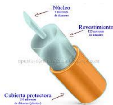
Figura 8 Fibra Monomodo (SM)
