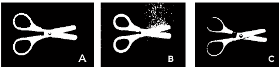
Figura 31: A: umbral óptimo 97, B: umbral = 45, C: umbral = 140
