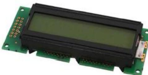
Fig. 3.25: Pantalla LCD 2x16. (FUENTE – basic.pdf, 2011.)
