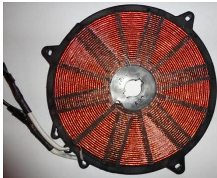
Figura 25 Inductor resonante
