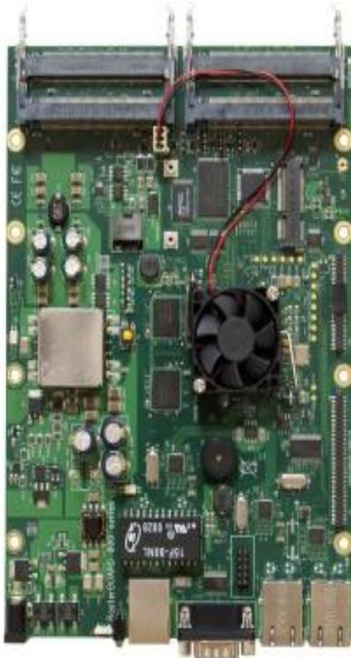
The RB800 is an advanced high performance wireless platform. It has four miniPCI slots, three Gigabit ethernet ports, two daughterboard connectors, a miniPCI-e slot and a compact flash slot.
