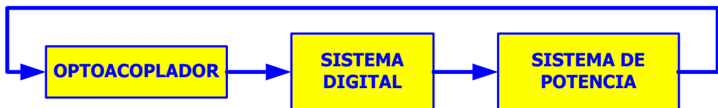
Figura 4.3 Bloque de control PLC
